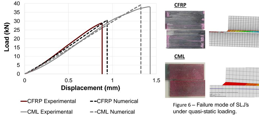
Figure 7 – Typical load-displacement curves of SLJs under quasi-static loading.
