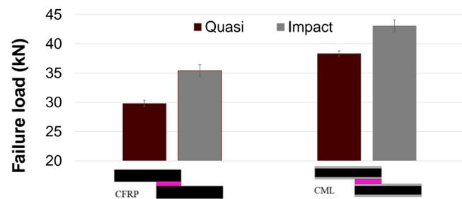
Figure 10 – Effect of strain rate on failure load.
